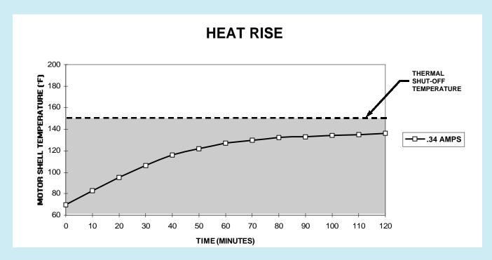
All of the pump models in the Performance Data and Heat Rise charts are in the shaded area, meaning they are capable of sustaining continual running, at any of the above listed pressures, without shutting down to allow the motor to cool. To conserve wearing parts, however, the pump should only operate as needed.
